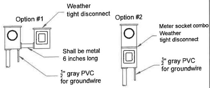
Grounding bushings shall be installed on metal nipples in the meter socket and panel box.
